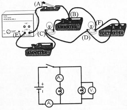
18) Label all the points indicated on the schematic diagram, on the circuit picture.
